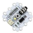
On-board there is a PICAXE 14M2 programmable IC, a dimmable white LED, a momentary push switch, a 3.5mm stereo socket for ease of programming, and a JST connector for attaching a battery pack. There are also 6 sewable I/O pins, making this a really versatile control board. Pins C0, C1, B5, B4, B3, B2 (the on-board LED) can be used to fade LEDs (using Pulse-width modulation) and Pins C0, C4, B5, B4, B3 can be used to read analogue inputs.
