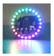
Programming the ZIP LEDs is easy using the Microsoft MakeCode Block editor.
