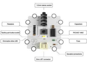
It can be powered either by the JST connector, or the clearly marked '+' and '-' connections via conductive thread, from a power source between 3V and 5.5V.
