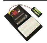
This is a great way to start making circuits and making experiments. It gives access to the pins on the bottom of the BBC micro:bit using our specially designed Edge Connector Breakout Board. This is used in conjunction with a Small Prototype Breadboard which makes it easy to connect additional components using the included jumper wires. No soldering required.
