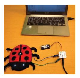
Clip leads can be used to test designs
