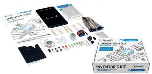
It contains everything you need to complete 10 experiments, including using LEDs, motors, servo motors, light sensors and capacitors. The easy to follow tutorial book guides the user through everything they need to know about programming an Arduino microcontroller.
