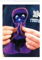
↑ Examples of conductive fabric used on the hands of puppets. When these are touched together, the circuit is completed and the LED lights up.
