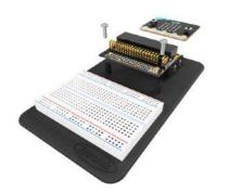
The assembled Edge Connector Board.
