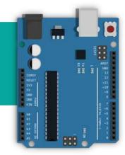
The Arduino is controlled by the code with which it is programmed. This code is written in the Arduino programming language, using the Arduino development environment. Once complete the code is easily programmed on to the Arduino board using a simple USB lead.
