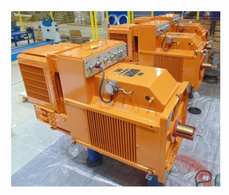
Ambient temperature: -40 to +55°C CSA certificate: Class I, Div 2 Groups A,B,C,D Insulation class: H Power supply via frequency converter Forces ventilation: 50 Hz ili 60 Hz
