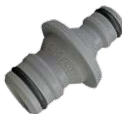
art. 4433 niplex with high flow male coupling (15 mm Flow) and 1 standard male coupling (9 mm Flow) To connect the "professional" system to the "standard" one
