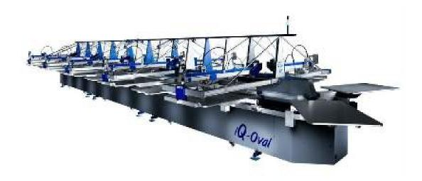
A 100% registration accuracy is provided by having each printing station it's own pin, sothere is no part which will stretch and loose this accuracy. The iQ-Oval is equipped with the latest "m-touch pro" operating system with tablet interface. It has the widest pallet printable area of 90 X 110Cm up upto 9 Colours. This gives a fast and accurate print productivity act.
