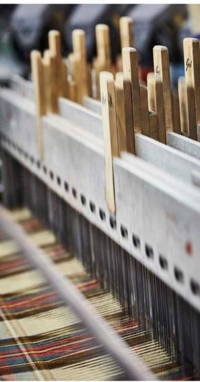
These are the first stages of the production process where the intricacy of the final design begins to show. Taking our mélange yarns, we vertically align up to 6,000 threads in the warp.
