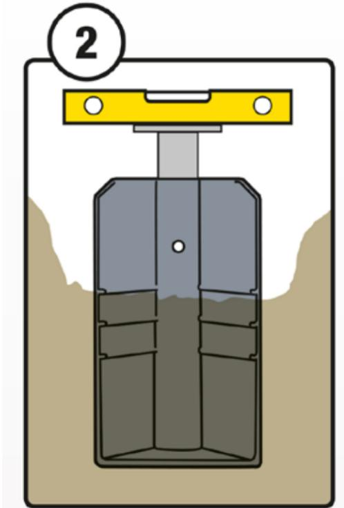
2. Place the base into the hole and fill it back up with soil until the upper stripe. Level the base, press the ground firmly and water it.
