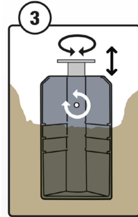
3. Adjust the height and direction of the mounting plate and fasten with the bolt.
