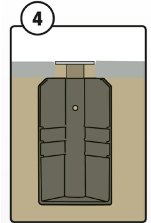
4. Fill the hole completely, press the ground firmly and water it again.
