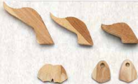
Roughly cut & sanded feet
