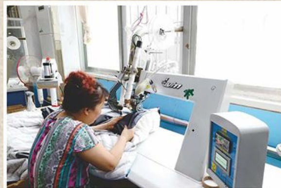
Hot air seam sealing machinery
