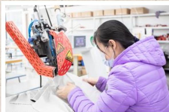
Hot air seam sealing machine
