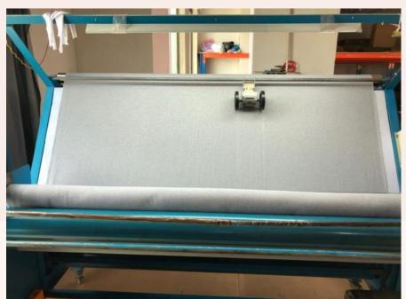
By mechanical rolling of fabric with adjustable speed control, the staff can easily inspect the quality of fabric to avoid any possible shade difference or defect, while fabric length is also measured in the same process.
