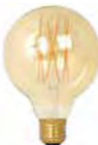
8. LED Filament Globe Gold Finish CAL-425464. ES, G95 (Globe) 95 x 140mm. Efficiency A+; 4W; 320 Lumens; 2100 Kelvin; Dimmable
