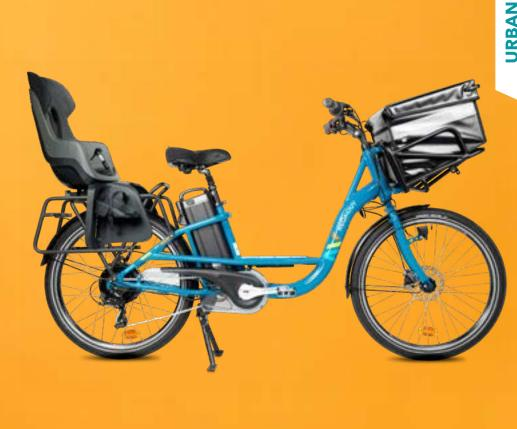
Our utility bike is designed to carry large loads via its front and rear luggage racks. Getting on the bike and setting off when fully loaded is easy thanks to its low step through frame and start assist trigger.
