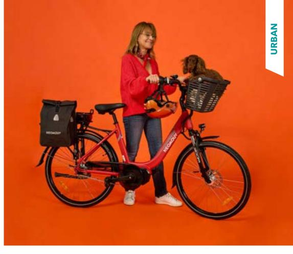
The KALYSO 2 HY N7 is equipped with a central motor and an internally geared rear hub by Shimano to prevent derailment of the chain and facilitate gear changes even when stationary.
