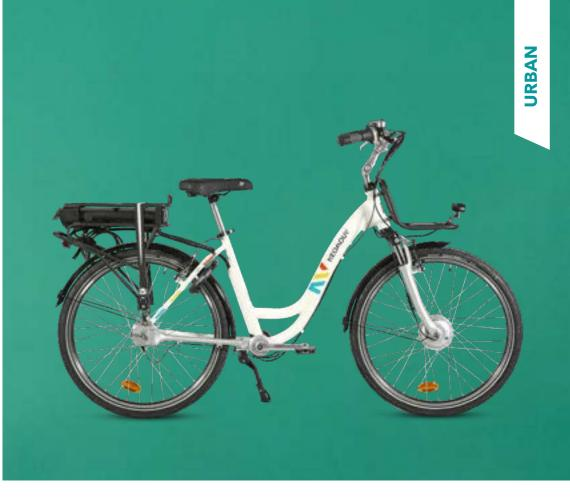
Our fleet bike is equipped with a Cardan shaft transmission for ease of maintenance whilst avoiding chain derailment. It also features a front luggage rack capable of carrying loads up to 10 kg.
