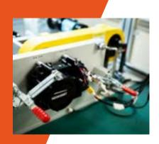
NEOMOUV now has two test benches for our engines. Allowing us to replicate real-world and extreme usage to ensure long term reliability.
