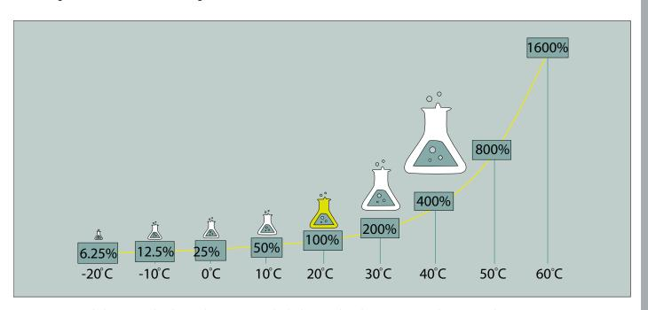
At temperatures below 20°C, the chemical processes inside the battery slow down. Assuming that 20°C is the optimum temperature for 100% performance, the chemical reaction speed and starting performance drop to 50% at 10°C. At freezing point, battery performance drops further to just 25%.
