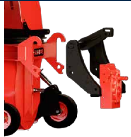
Can be pulled or pushed as standard. By using a gear-box-kit it can also be mounted in front of the tractor
