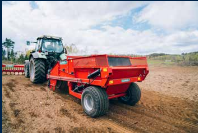
Wheel axle with hydraulic lift gives a tipping height of up to 2.5 m.
