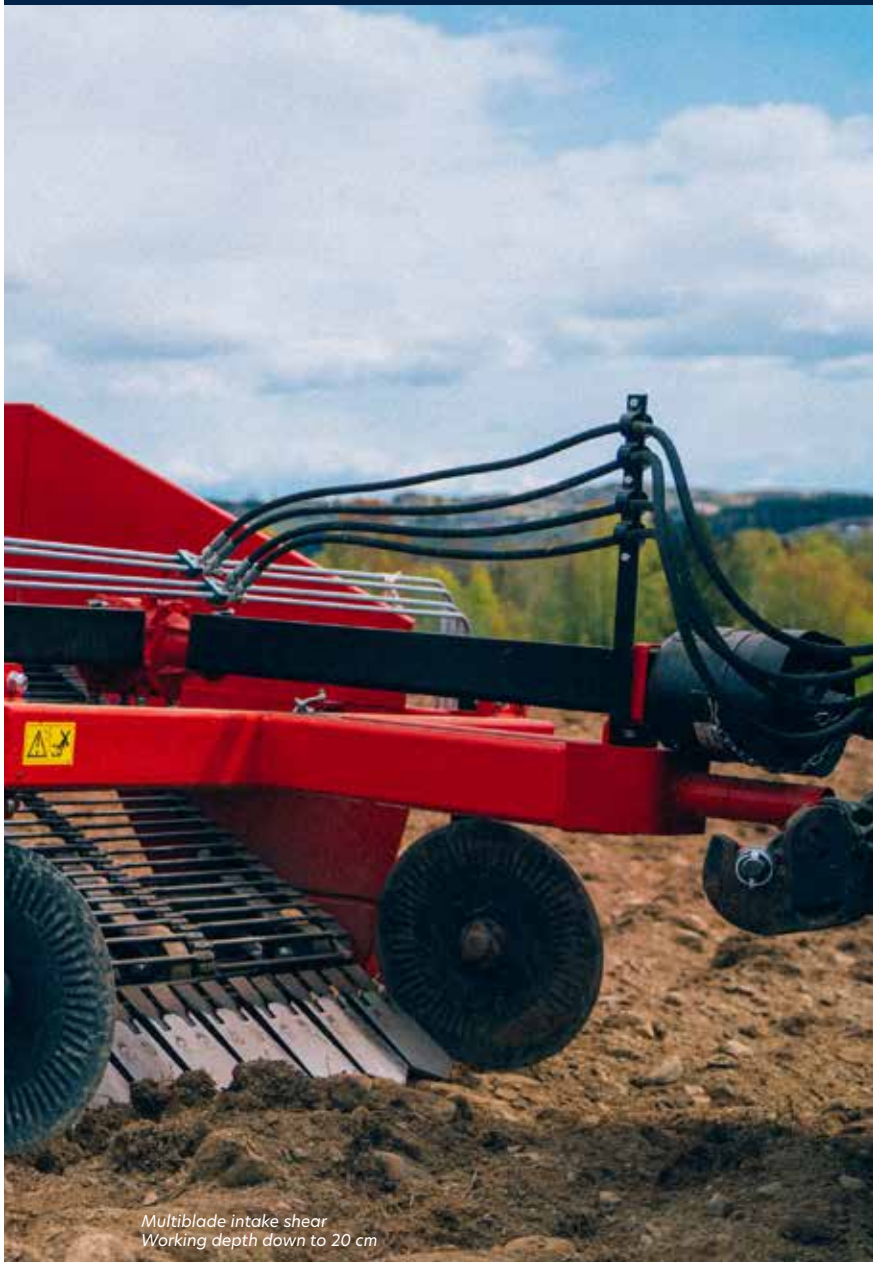
Different spacing on web bars. From 16mm up to 44mm.
