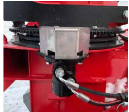
Chute rotation: New larger 50cc hydraulic motor
