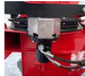
Chute rotation: New larger 50cc hydraulic motor
