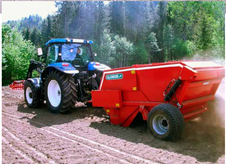
Wheel axle with hydraulic lift gives a tipping height of up to 2 m.
