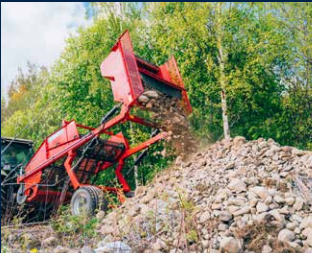
Wheel axle with hydraulic lift gives a tipping height of up to 2.5 m.
