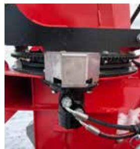
Chute rotation: New larger 50cc hydraulic motor.
