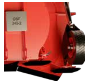
Two skid shoes at rear, next to the impeller house: providing excellent float and perfect adaptation to the ground.
