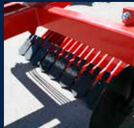
Different spacing on web bars. From 16mm up to 44mm.
