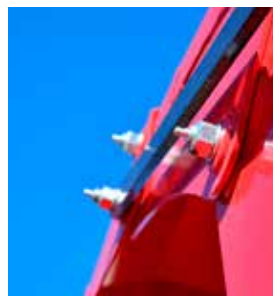
Grease Fittings on all links of the Chute deflector.
