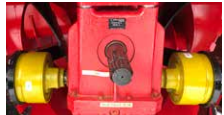
Large solid gearbox and automatic overload device on intake auger.
