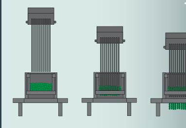
The bulk sample of peas is compressed and sheared, accurately simulating the bite and chew mechanism
