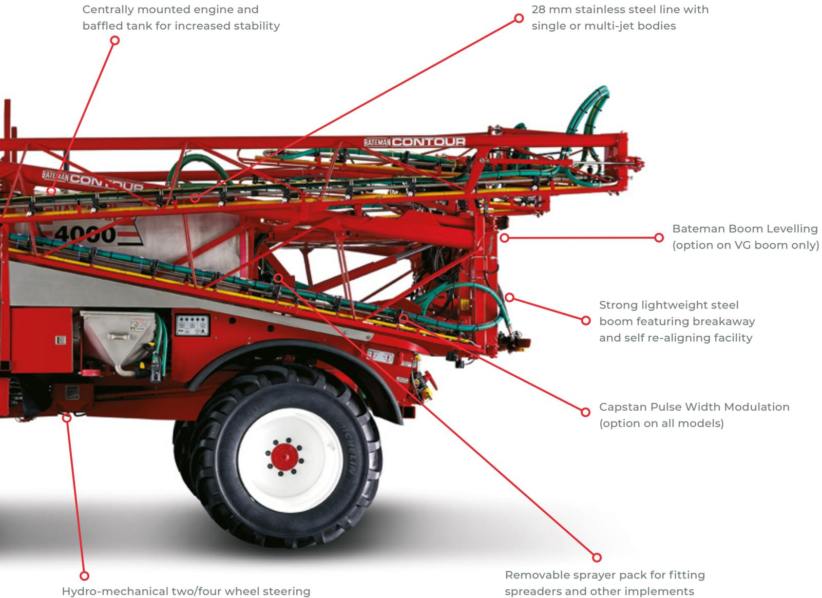
Centrally mounted engine and baffled tank for increased stability
