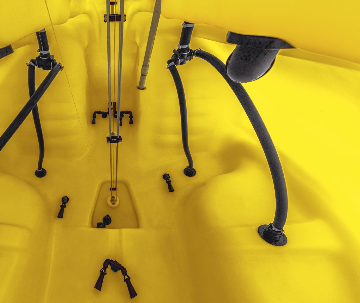
A look inside the tank of the R900i shows where AutoDilute and Continuous Dilute work.
