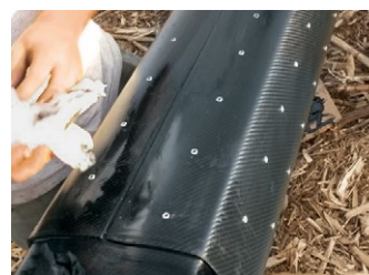
With the new carbon layers glued and riveted in place, the repaired boom is again ready for duty in the field.
