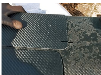
New Carbon Fibre sections, supplied in the repair kit, are cut to the profile of the damaged boom section.
