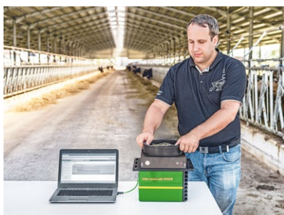
Use of the HarvestLab™ 3000 as a stationary laboratory to determine feed rations.
