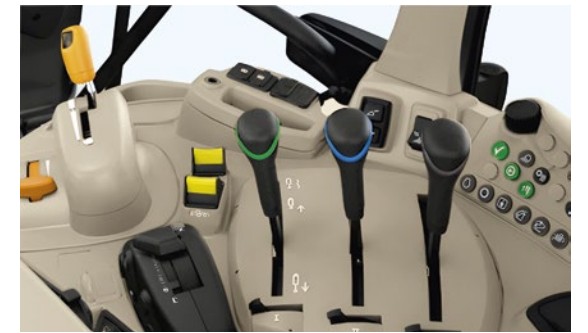
AutoPowr™ on the right-hand console with mechanical SCVs
