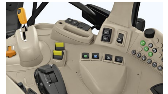
AutoPowr™ on the right-hand console with electrical SCVs
