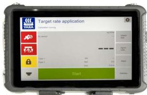
All new N-Sensor installations come with a tablet PC which runs the software and links to the rate controller. This tablet records Biomass and N applied maps (in most cases).
