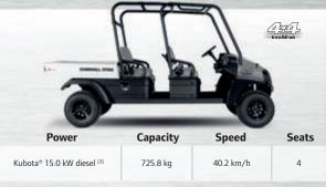
system and four forward-facing seats, this vehicle carries two crews and their gear, even over rough terrain.
