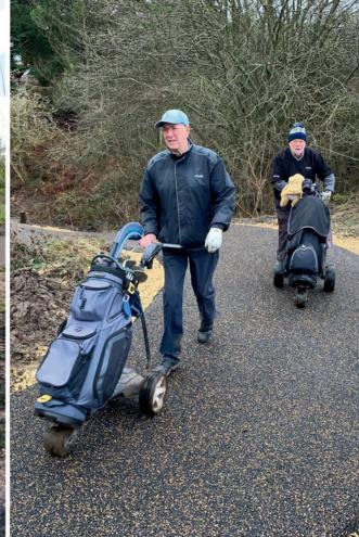
Flexipave is a mixture of loose ground rubber (derived from recycled vehicle tyres) and stone aggregate. The loose material is mixed onsite with our unique polyurethane binder and installed by hand.
