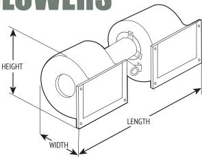
Use the diagram above as a reference to measure the dimensions of your blower. This will help you determine which is suitable for your vehicle.
