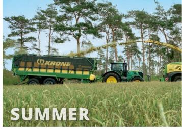
Whole crop silage The articulated drawbar lowers the front end for easy filling from the forager.
