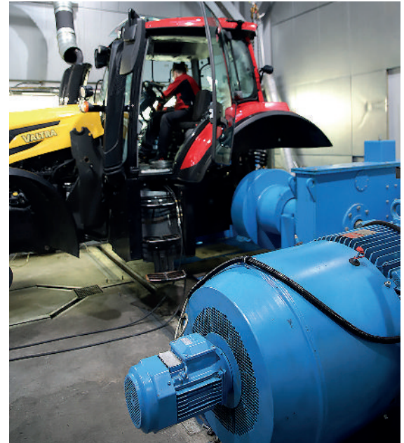
Jan-Erik Karjula operates a tractor on the testbed. The results will be used to further develop both the tractor and the simulator.
