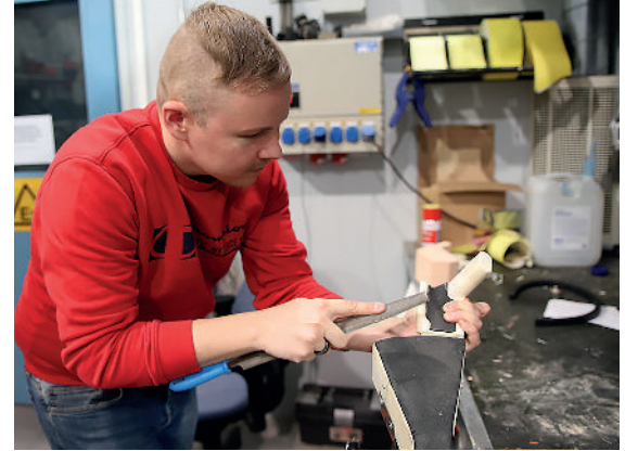
Industrial Designer Henri Hokkanen works on a plastic model of an armrest. A lot of plastic, wood and 3D-printed components are used in the design studio to make full-size mock-up models of future tractors and cabs.
