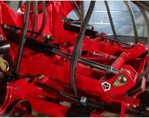
*Six degree wing pivot for ultimate contour following and seed placement*
