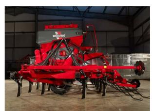
*Four rows of tines for high trash clearance*
