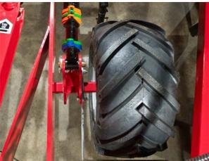
*Hydraulic depth wheel with aluminium spacers*
