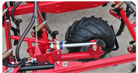
Manual Depth Control with aluminium spacers
