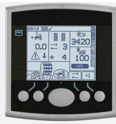
RDS Artemis Lite Controls for GPS forward speed monitoring
