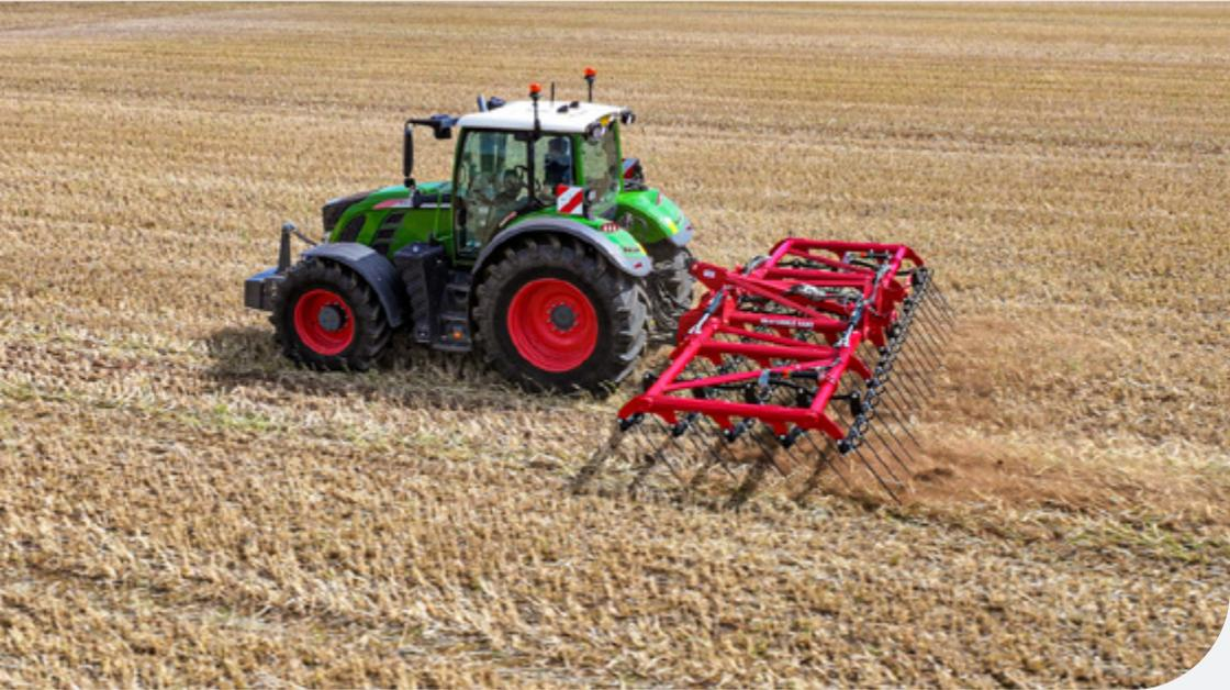
With its unique tine configuration and design, the Weaving Stubble Rake is able to create ideal conditions in which weed-seeds and volunteers will readily germinate allowing for control before drilling. This machine is able to decimate slug eggs and weeds including black grass in growing crops. The Stubble Rake is used at high speeds and is able to work over a large acreage in a short amount of time.
