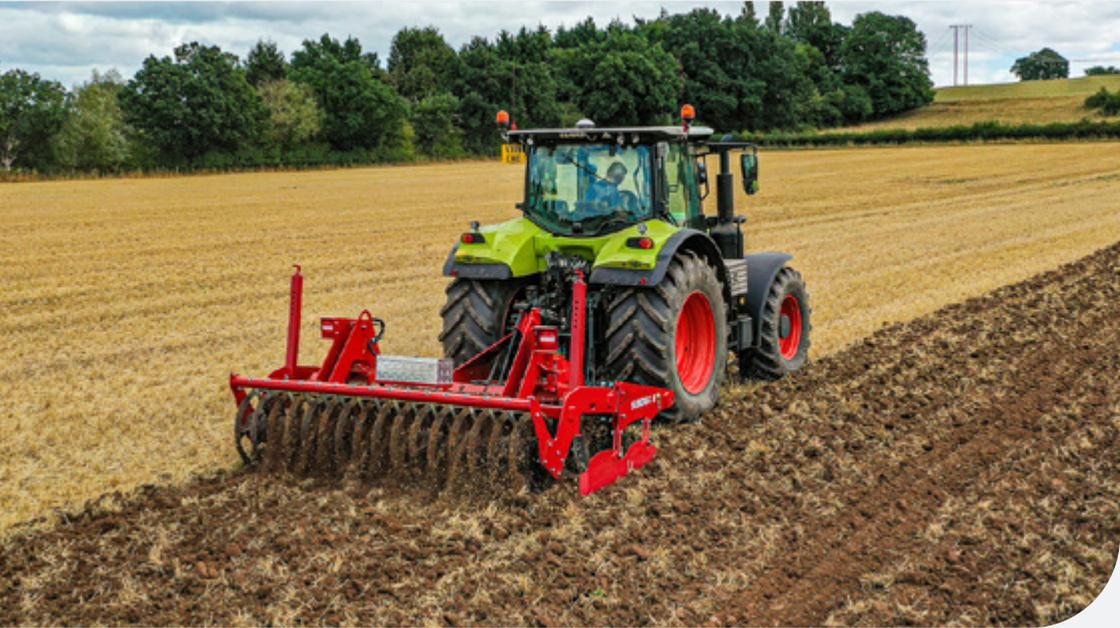
The low draft legs are designed to break up the soil pan and aerating the soil without creating much disturbance to the soil surface, whilst the discs are able to chop and mix crop residues and create a stale seedbed, with the packer roller leaving a level finish.
