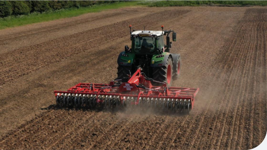
Working depth is between 0 and 15cm (6"). 167mm spacing between legs is similar to our Sabre drill allowing for high volumes of trash to flow through and ensure all ground is worked.
