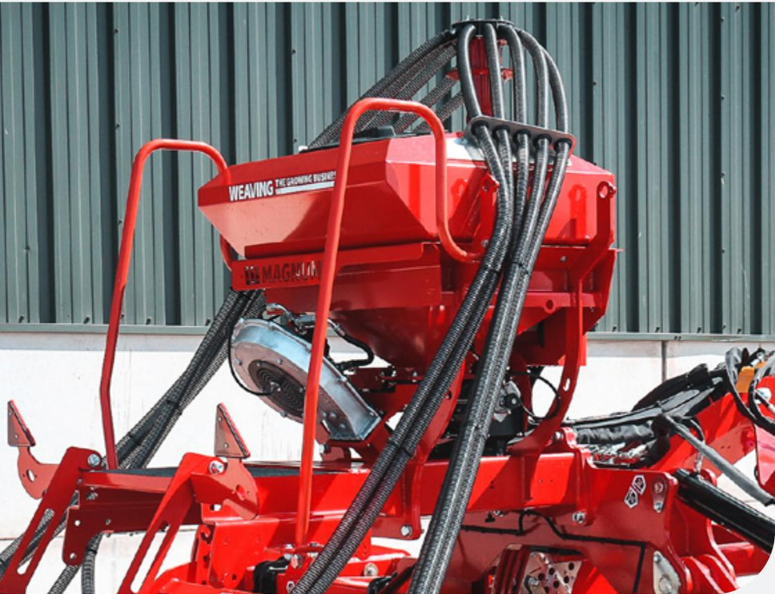
Fitted with an Accord pneumatic distribution system, it is suitable for sowing oilseed rape, grass, cover crops, slug pellets and a wide range of seeds up to 12 metre working width.
