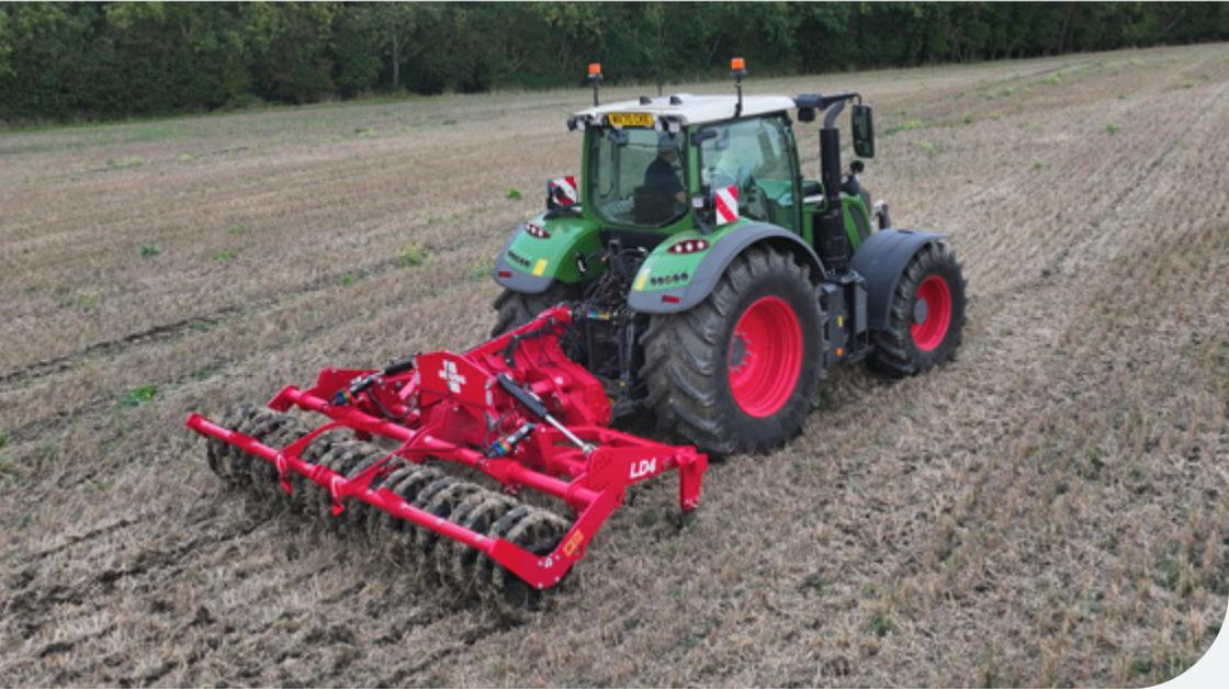
The ultra-low disturbance heaving action of the LD Top-Soiler relieves compaction in the top 9" (228mm) of the root zone, providing soil aeration and better water infiltration, while leaving the soil surface virtually undisturbed. The legs are followed by a heavy duty cast ring roller which leaves an even surface finish.
