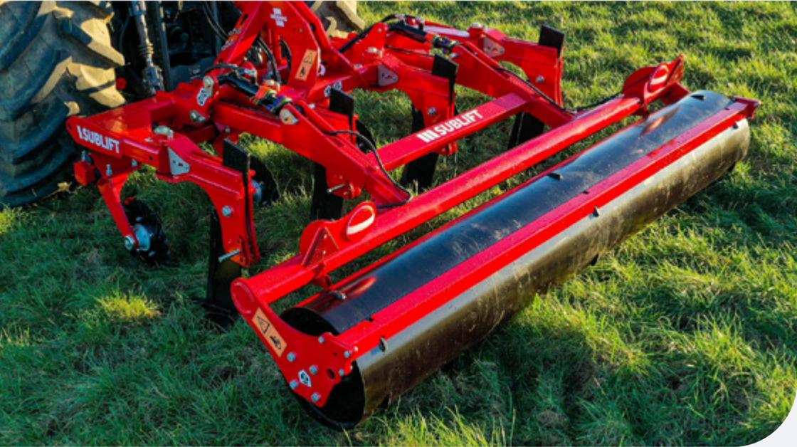
Designed to manage soil compaction issues caused by heavy machinery and grazing livestock that can often result in waterlogging and poor-quality pasture.
