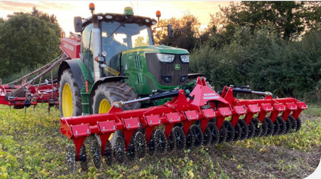
With front linkage mounting and a full width set of wavy discs, it is able to cut through trash and cover crops in front of the drill, clearing the path for the drill to both improve seed to soil contact and prevent debris from hooking around the coulters and causing blockages.
