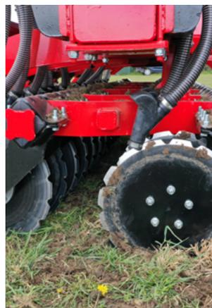
2 Rows of Serrated Discs on Rubber Torsion Bars
