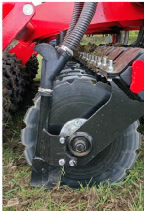
Hardened Seed Tube with Weaving Rubber Exhaust Boot
