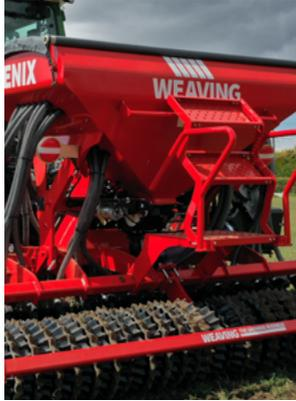
*Folded rear loading step with a security hand-rail & LED road lights*
