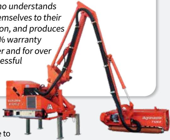
Each flail mower in the Agrimaster range is equipped with a unique cutting action with a throw over the back roller technique to level a clean and level finish and a fine residue which will break down faster.
