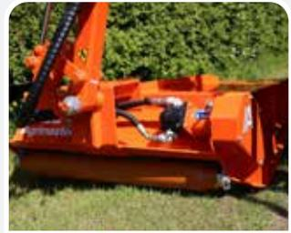
Dual Direction Rotor/Cutting Head
