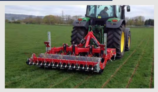
The GLS grassland sub-soiler is designed to alleviate subsoil compaction by opening the sward and lifting the soil to improve drainage and airflow.
