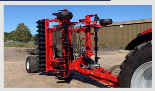
The LDS alleviates subsurface compaction with minimal surface disturbance, creating a well structured, aerated and free-draining soil.
