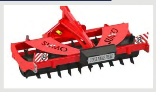
The Sumo Front Grassland Aerator opens up the grassland sward to alleviate compaction, allowing air to flow through the grass roots, letting nutrients enter the soil and aid drainage.
