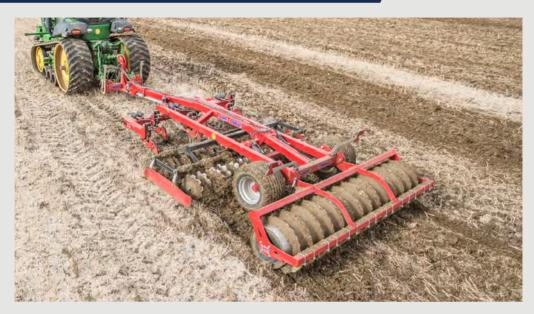
The TRIO trailed combination cultivator works the whole soil profile in one pass and can be used in most instances instead of the plough.
