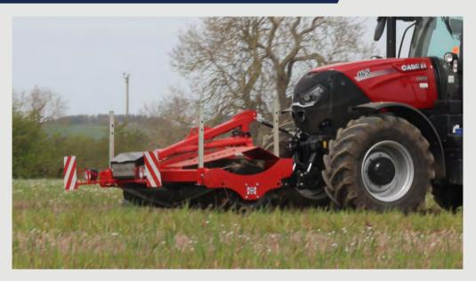
The Crimper rolls and breaks cover crops, preparing the field ahead of drilling, reducing reliance of herbicides.
