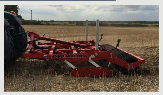
This MULTIPRESS cultivator is designed to till, level, and press on ploughed, cultivated soil or stubble before the drill, leaving a weatherproof surface.
