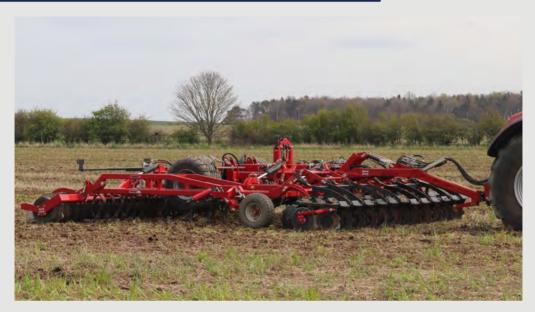
The VAXIO is a high-speed and versatile cultivator which combines both surface cultivation and loosening at depth, with levelling and consolidation all in one pass.
