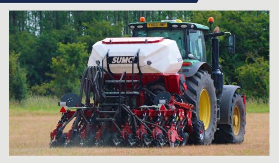
The DD system is a zero-till system, crop residues left in the field are incorporated into the soil by the DD coulter as it places seed in the ground.
