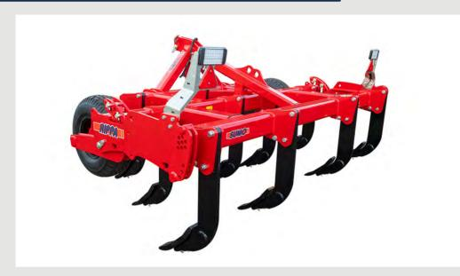
The RIPPA effectively revives saddened or slumped soils via an arrangement of aggressive tines. Aerating, the soil prior to planting can encourage root growth, improving the flow of oxygen and nutrients through the soil and help prevent future runoff.
