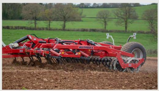
This MULTIPRESS cultivator is designed to till, level, and press on ploughing, cultivated soil or stubble before the drill, leaving a weatherproof surface.
