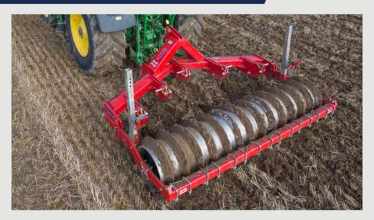
The heavy-duty SUBSOILER can work deep to lift the deepest of compaction layers caused by heavy traffic, wet season or poor cultivation techniques.
