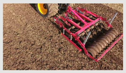
The TRIO mounted combination cultivator works the whole soil profile in one pass and can be used in most instances instead of the plough.
