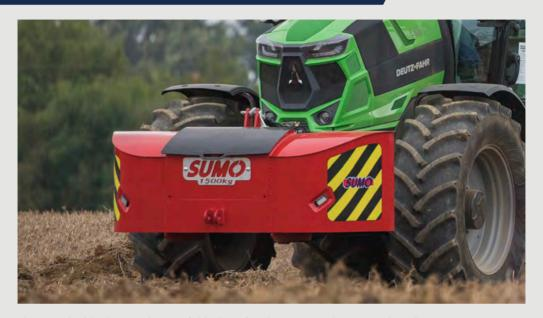
The Weight block provides useful ballast for the tractor, the integral toolbox can carry many anything from tools to wearing parts, providing a much-needed place to store cab-floor clutter. Weight blocks are finished in red & black and feature an internal toolbox, tool tray, high visibility
