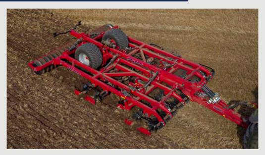
The QUATRO trailed combination cultivator works the whole soil profile in one pass, ideally suited to trashy conditions.
