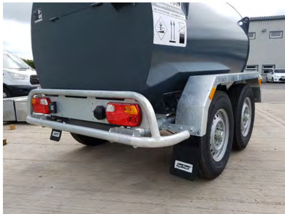
HIGHWAY COMPLIANT LIGHTING / TOUGH, GALVANISED MUDGUARDS
