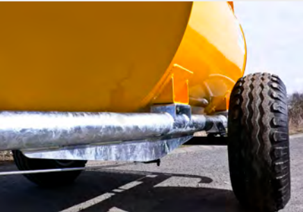
REINFORCED GALVANISED TUBULAR STEEL CHASSIS FOR EXTRA STRENGTH AND DURABILITY
