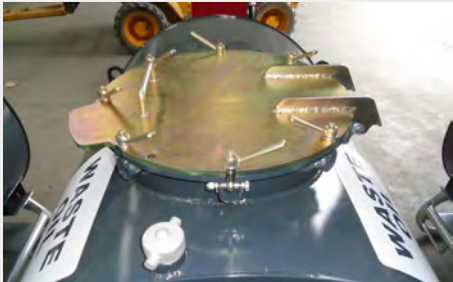
MANWAY FILLING POINT WITH SECURING POINTS AS STANDARD
