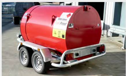
HEAVY-DUTY GALVANISED STEEL CHASSIS
