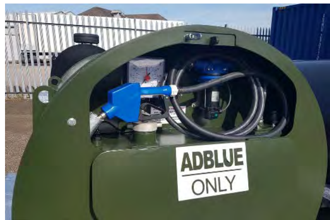
HYDROSTATIC CONTENTS GAUGE ON ADBLUE TANK FOR LEVEL READING
