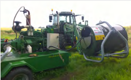
TANK CAN BE LIFTED AND MOVED EASILY BY ANY MACHINE WITH A 3 POINT LINKAGE
