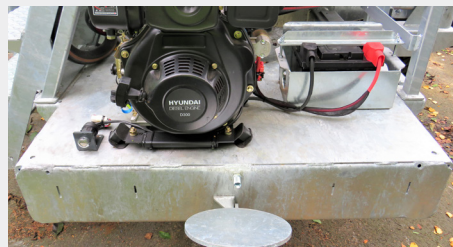
DIESEL ENGINE PUMP AND WATER OUTLET AT REAR WITH ADJUSTABLE SPREADER PLATE; SPRAY 6M
