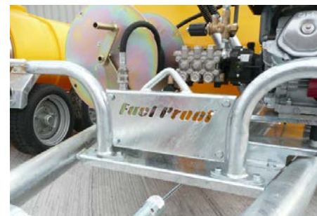
HAND REWIND HOSE REEL WITH MAX. CAPACITY 50M X 3/8" HOSE
