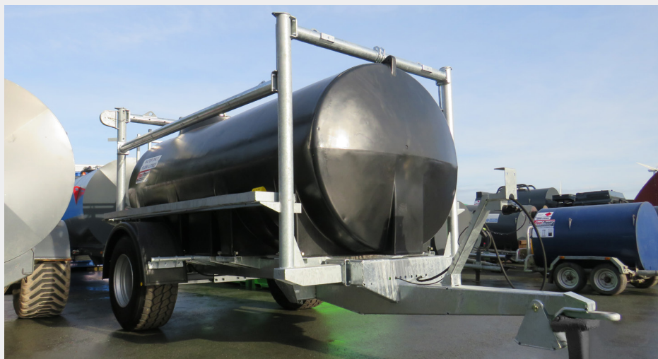
10,000 LITRE DUST SUPPRESSION WATER BOWSER WITH 70L/MIN FLOW RATE; SPRAY TIME 2 HOURS 20 MINS
