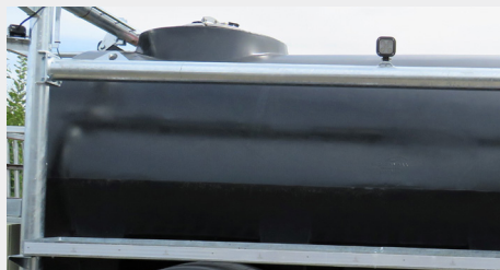
MANWAY ACCESS TO TOP OF TANK FOR MAINTENANCE AND CLEANING; SECURE LOCKABLE LID
