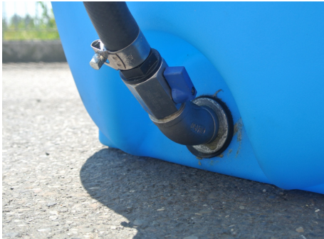
DISPENSING HOSE OUTLET CONNECTION POINT
