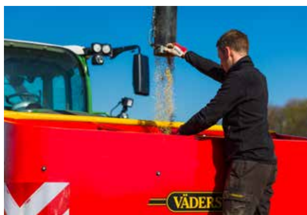
The sloping front design gives the driver good visibility. The wide opening and built in step makes it easy to fill.
