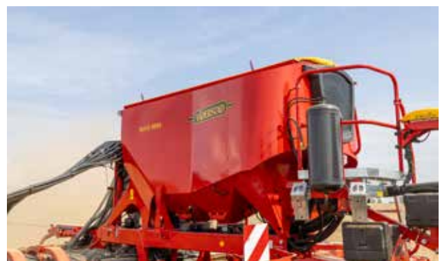
The seed-only model Spirit 600-900S holds 5000 litres.
