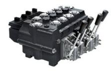
Load independent proportional valve with flow up to 180 I/min [48 gpm] and pressures up to 350 bar [5076 psi].
