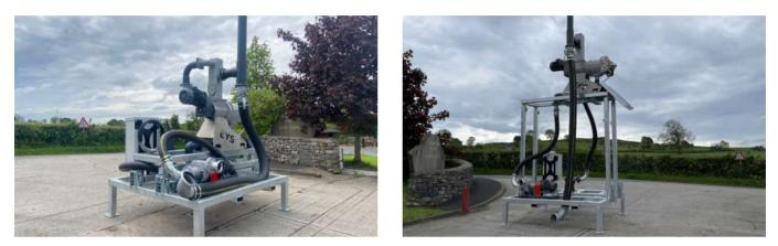
Storth keep things as flexible as possible with the choice of long shaft, submersible or Positive Displacement (PD) feed pumps. A stone trap is incorporated into models where longer distances require the PD pump, this avoids potential damage and breakdown. In general, the proven Storth long shaft pumps are the most popular due to their simplicity and external slurry electrical motor operation. In all cases the skid unit has pump storage capability for mobile transportation.
