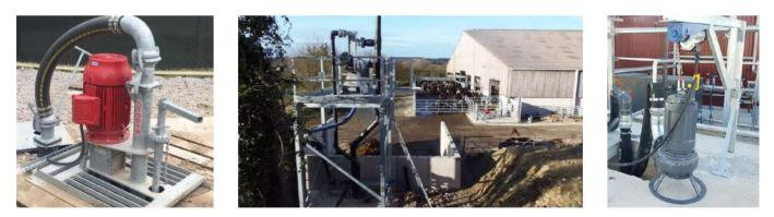
5.5kW to 22kW pumps are available in a range of formats to suit specific farm requirements. The most popular is Storth's own long shaft "Superjet" pump. However, certain sites may be more suitable for the Storth-EYS submersible pump or even piston pump.
