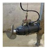
To achieve efficient separation, it is beneficial to present separators with a consistent Dry Matter (DM) slurry. Therefore prior to engaging the separator, slurry is often premixed. Storth can achieve this in a few individual ways with long shaft surface mounted mixers, submersible mixers or long shaft pumps in mixing mode, all of which are 3 phase electrically powered.
