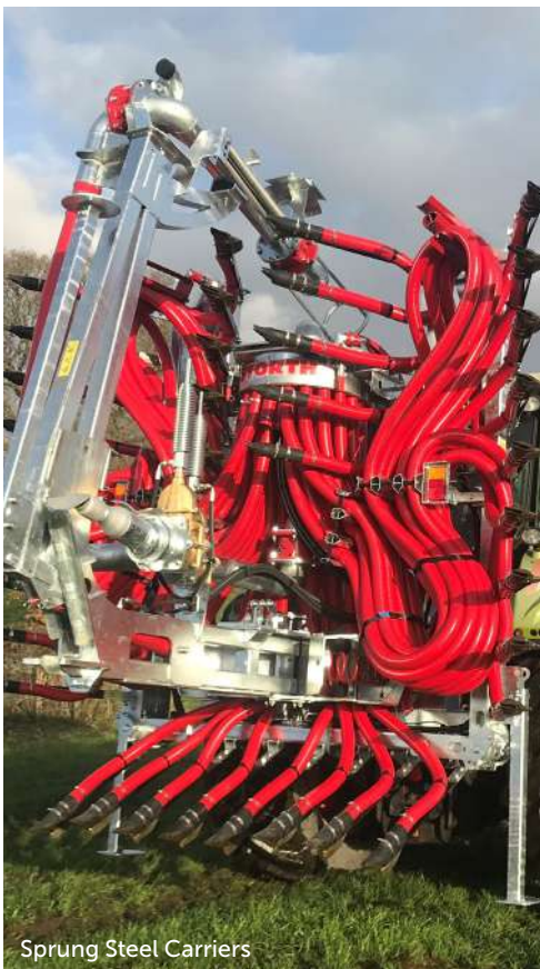
9m Contractor Trailing Shoe
