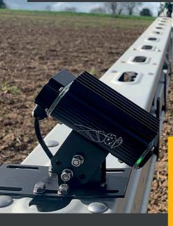
The Controller receives the information from the sensors and merges it to control the spraying and create the map in real time. Infestation and treatment maps could be exported at the end of the treatment and are reported in real-time to ISOBUS TC server.
