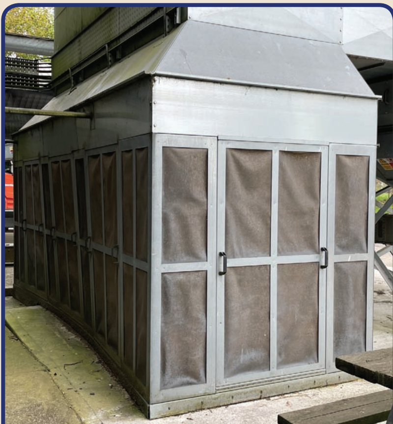
Optional Furnace Mesh Enclosure, for use in dirty environments where there is a lot of chaff to prevent accidental fire.
