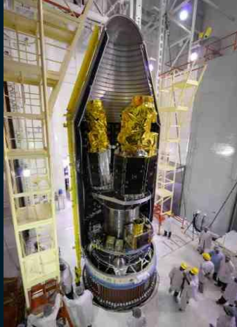
3x EO minisatellites constellation – launched in 2015 7-year op lifetime 1-m GSD (0.85-m) pan, 4-m 4-band m/s, 3000km swath length
