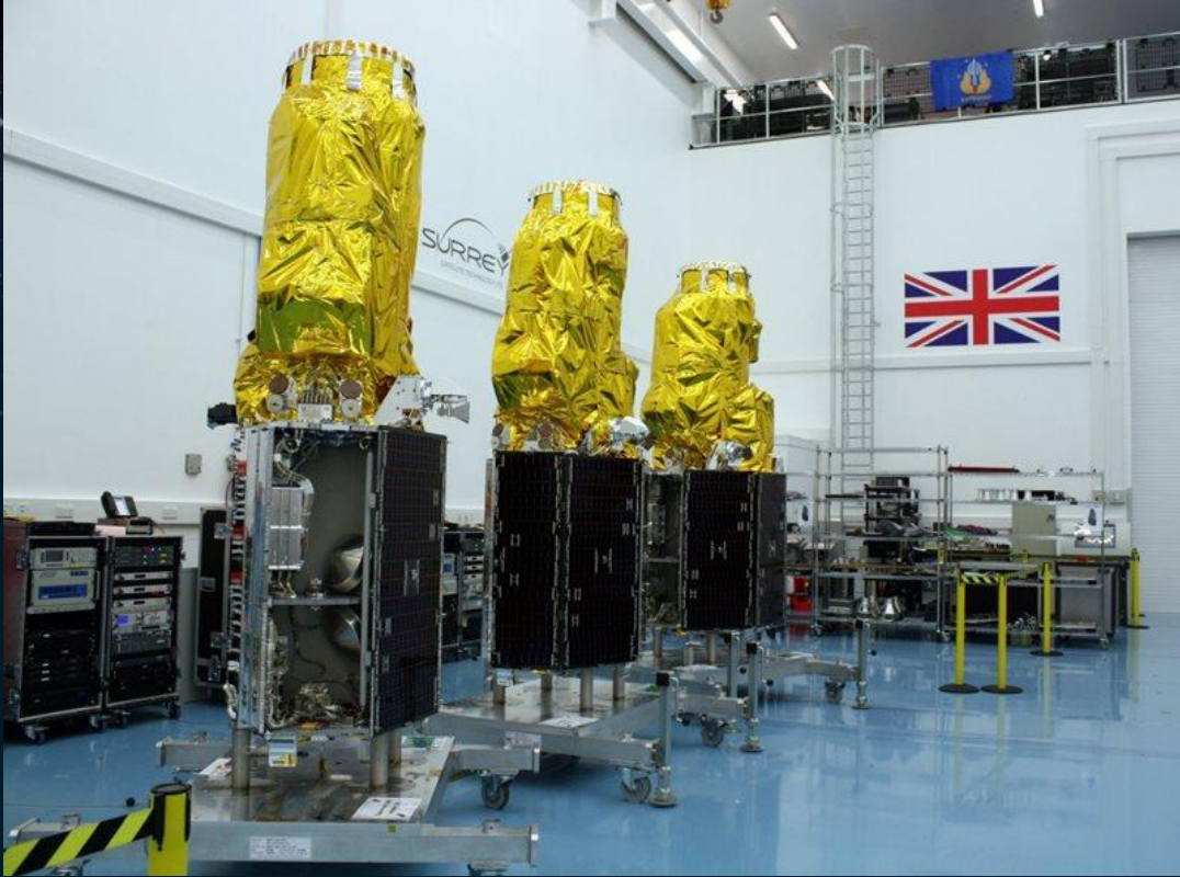
3x EO minisatellites constellation – launched in 2015 7-year op lifetime 1-m GSD (0.85-m) pan, 4-m 4-band m/s, 3000km swath length
