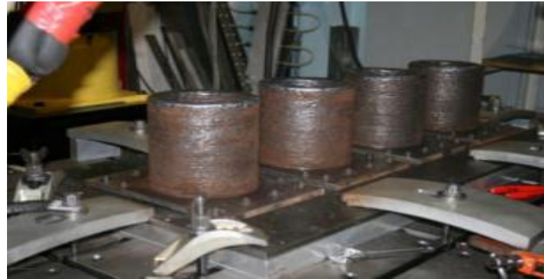
Mass 32 kg each // Deposition rate 4 kg/hr
