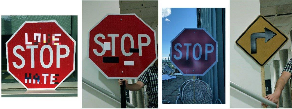
Subtle perturbations cause a neural network to misclassify stop signs as speed limit 45 signs, and right turn signs as stop signs.
