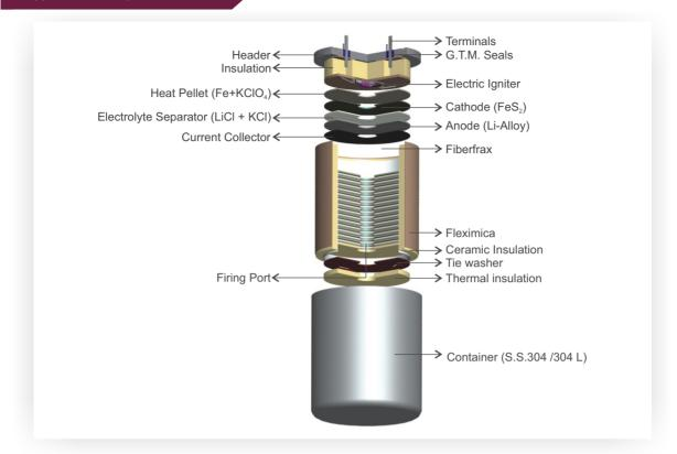
HBL Thermal Battery ranges from [5-150V]. We supply custom – built batteries. The technology is based on Lithium alloy and Iron Di-sulphide. The technical specifications of batteries are :
