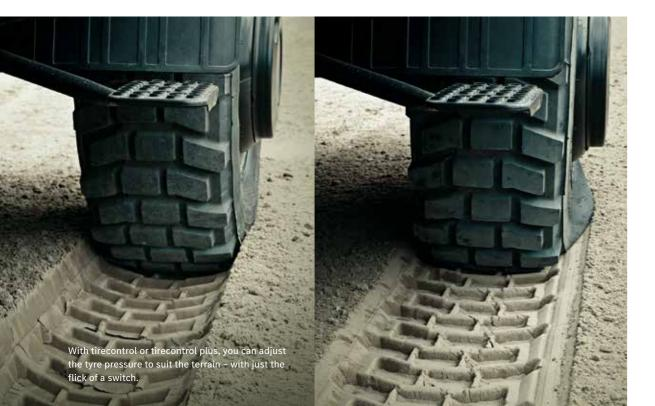
**Maximum traction for off-roading.** The tyre pressure can be raised or lowered using the tirecontrol or tirecontrol plus central tyre inflation system (CTIS) – separately, for front and rear axles, and to accommodate the current load and operating conditions. The result is high traction on any surface.
