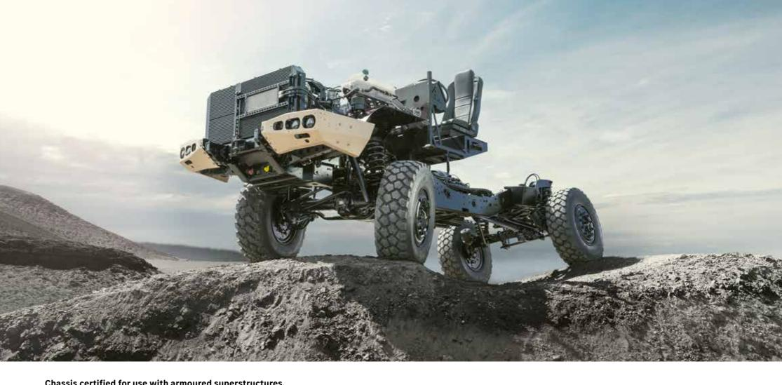
Chassis certified for use with armoured superstructures.
