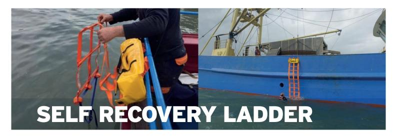
THE FIBRELIGHT SELF RECOVERY LADDER, BASED ON THE SOLAS FIBRELIGHT EMERGENCY LADDER, HAS BEEN DESIGNED AS A LIFE-SAVING DEVICE FOR FISHERMEN OPERATING VESSELS ON THEIR OWN OR WITH LIMITED CREWS.
