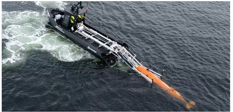
*Pictured: USV recovering the 780kg and 5.5m long HUGIN
