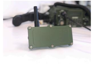
The Dismounted Officer Terminal (DOT) device is able to connect to a CNR radio (HF, VHF and UHF) to share voice and data services by means a wireless LAN (WLAN). The DOT device is able to create its own wireless network (access point) or work as a WiFi client.
