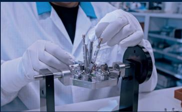
The size of parts and the required precision necessitate a controlled atmosphere in the entire assembly workshop, with continual air change and filtration. A clean room ISO 7 is
