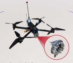
Equipped with light-sensitive camera with illumination for nighttime usage
